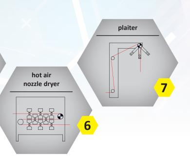
Terry towels are preferably printed with a weton-wet process. The chemicals required for reactive printing are applied trough a foulard or a MAGNOROLL-GMA applicator. The COLARIS is printing the design and passes the printed substrate on to the hot air nozzle dryer.
