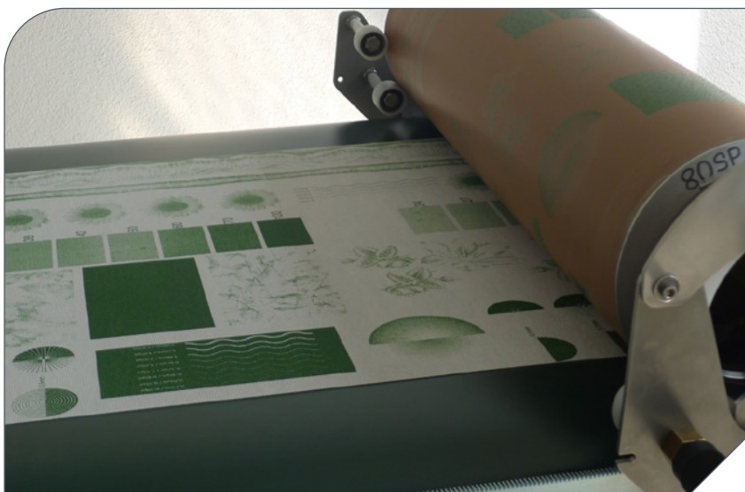
Mini-MD-R rotary screen sample printing machine
