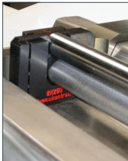
PVC coating with two roll rods
