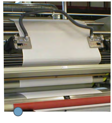
3 | The oscillating cloth pressure roller comes with a special silicon rubber coating surface, assuring to avoid cross marks on textile goods. The electronically controlled servo drive with automatic speed adjustment guarantees continuous oscillating roller movement without any stop ever.
