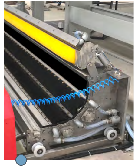
6 | Printing blanket washing device with high quality brushes and water recycling system for a minimum of fresh water consumption.
