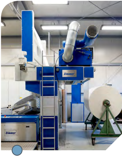
1 | The unbatching device comes with a stepless automatic digitally controlled speed control drive system, which transports any kind of woven and knits from small or large rolls onto the printing machine.
