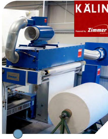
2 | Dust and lint removal device, new and improved, for most efficient fabric cleaning results. In various executions: brushing – suction – blowing with bevelled suction mouthpiece for one or both-side simultaneous cleaning of the fabric.
