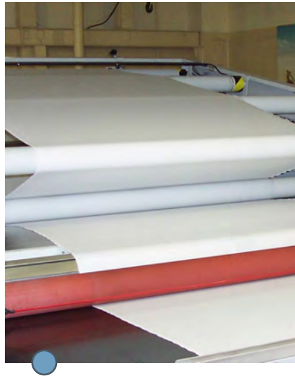
5 | Thermoplast glueing device with cloth heating shield and infrared heating elements. For perfectly uniform glueing of synthetic fabrics.
