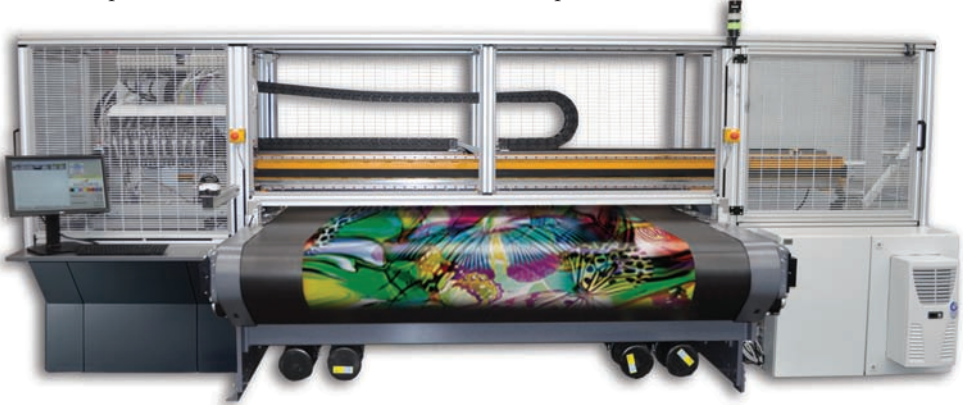
Zimmer Austria's six-color Colaris digital printing machines feature Fujifilm Dimatix StarFire™ industrial printheads and an "open-ink" system for flexibility in ink and dye choices.
