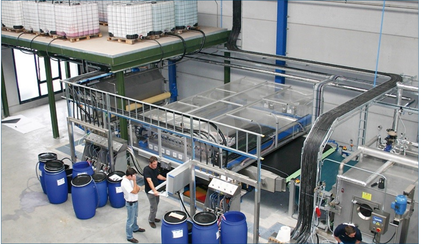
CHROMOJET 800 2000, with 12 colors / 256 jets per color and color supply tanks
