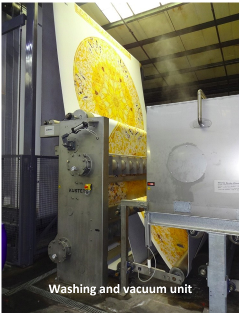
Steamer followed by washer and accumulator
