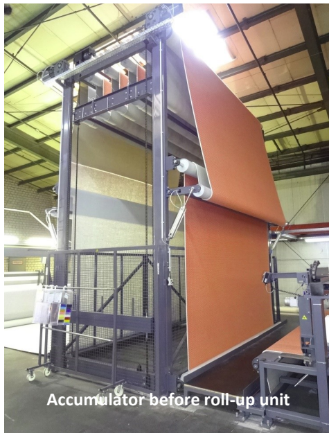
76 dpi print line at Maltzahn, Germany 420 cm width; 16 colors; 512 jets per color
