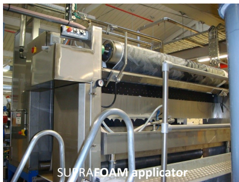
Carpet tile print line at Godfrey Hirst, Australia: 2,200 mm wide; 16 colors; 256 jets per color
