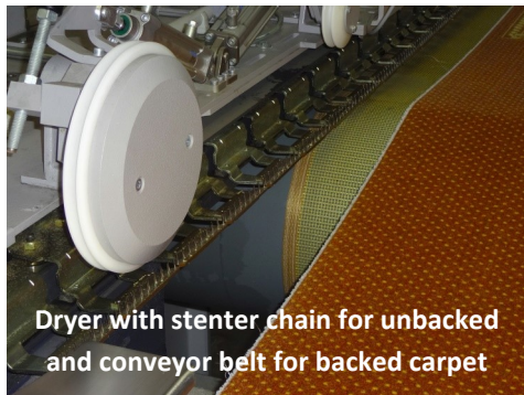
Center guiding followed by stenter dryer
