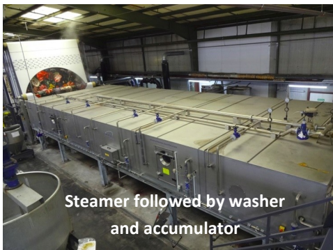
Unrolling, accumulator, pre-steaming, pre-washing, center guiding
