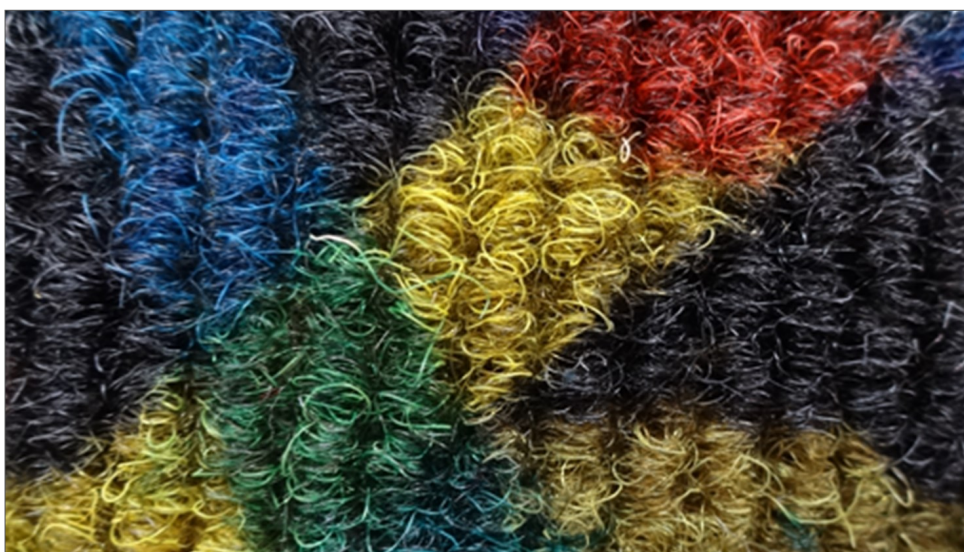
This picture shows a striped polyester needle-felt carpet printed on COLARIS using disperse inks, pressed by a SUPRAPRESS system and fixed by a HT steamer.
