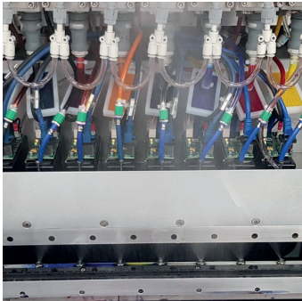
Automatic print head cleaning system
