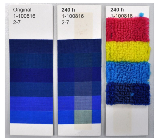
Lightfastness test on polyamide carpet
