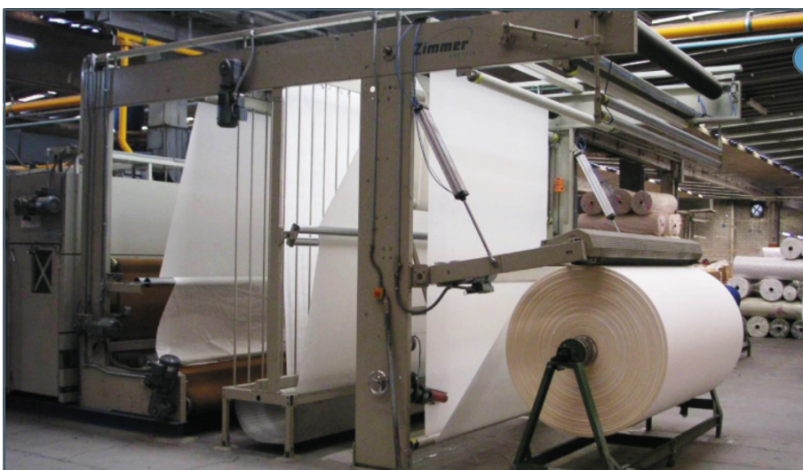
J-Box & re-batching arm
